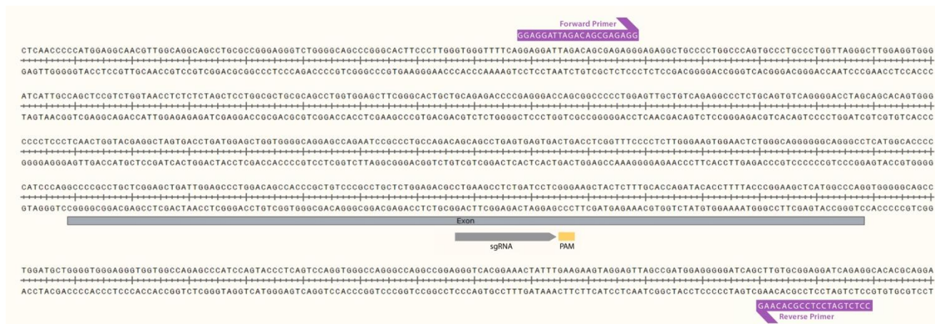
Figure 2. Sample primer design for amplifying the sgRNA target region. sgRNA target should not be positioned in the middle of the amplicon to show a discernible cleavage.
